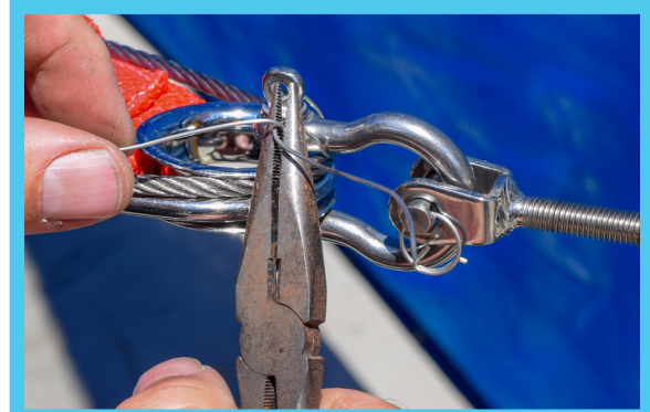
Twist the ends together to tighten the loop
