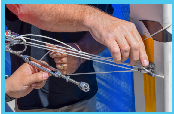
Loop the rope back through the D Ring and the attachment point multiple times.
