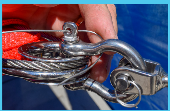
Feed Lock Wire through Bow Shackle pin and the Bow Shackle loop
